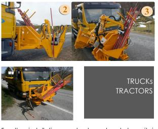
For the installation on trucks a bracket as it is needed for snow plows is required. A corresponding support must be present on tractors. Then it still needs a 24V power socket and 40L / 140bar hydraulic connector. Then your winter road marking work can be done fast and inexpensive!
